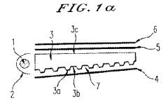
Figure 1a depicts a lightguide 3 having a primary light source 1, protruding trapezoidal patterns 3a, scattering reflection planes 3a and 3b, reflection sheet 4, and air layer 7. (Col. 4, ll. 51-67).
